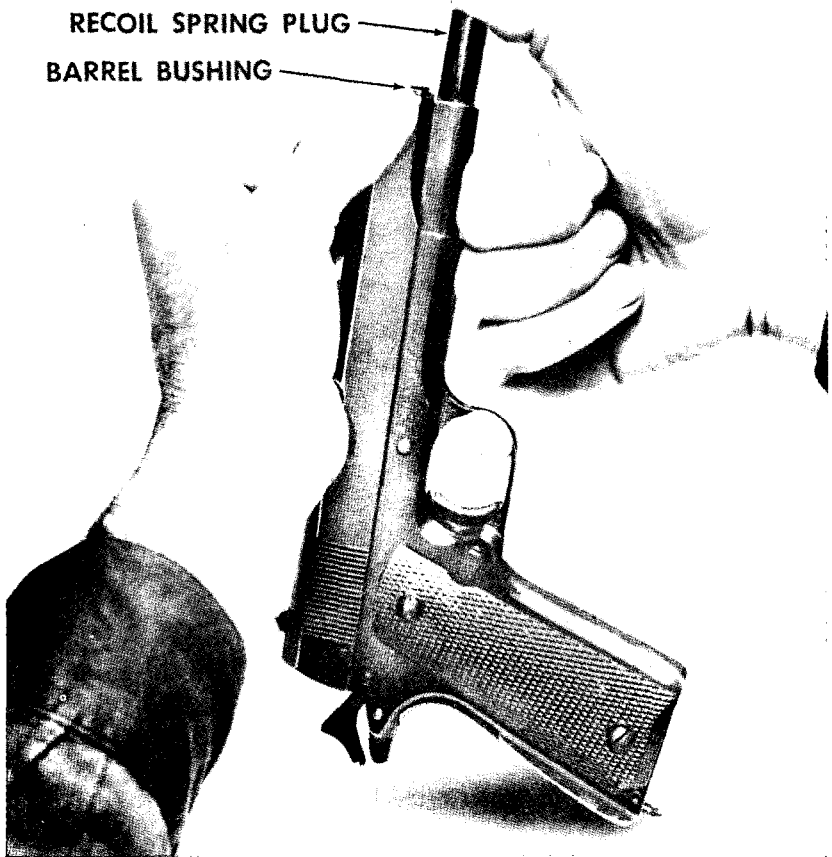
Figure 4. Press down on the recoil spring plug and turn the barrel bushing \frac{1}{4} turn clockwise. Allow the recoil spring to expand slowly, under control, to prevent injury or loss of the part. Turn the recoil spring plug counterclockwise and remove it from the recoil spring.
